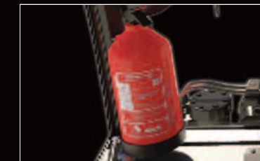
2 kg powder extinguisher
